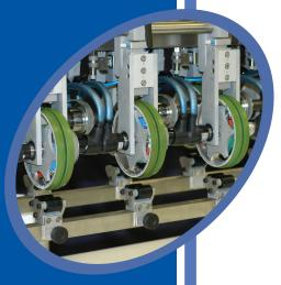
Continuous Rotary Heat (CRH) Sealing
