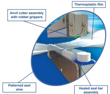
This seal is typically 1-1.5mm wide, showing a film material saving of approximately 10% against traditional crimp seals on the cross seal alone. The QPH sealing system ensures that heat and pressure are applied evenly across the sealing surface creating a completely fused, hermetic seal.
